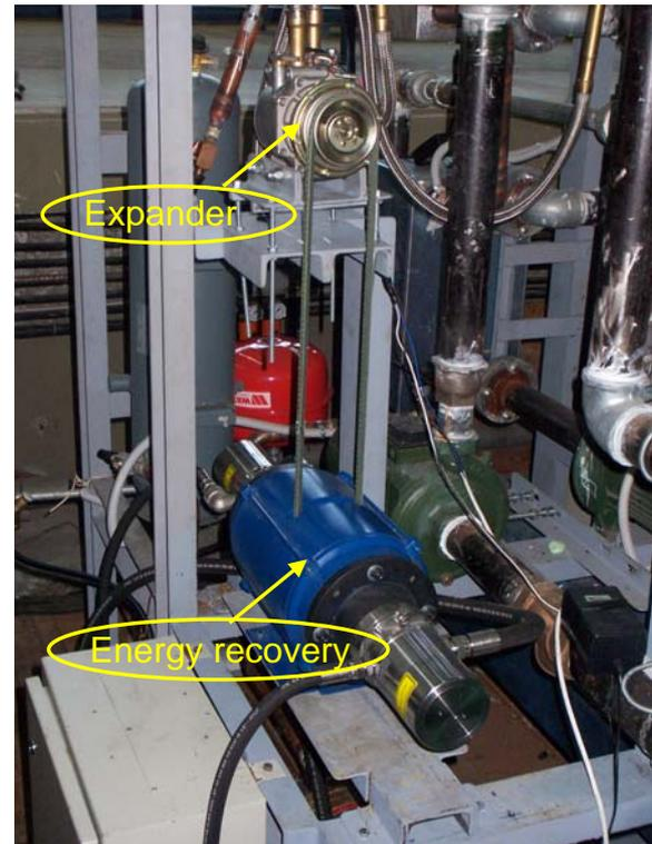
**Figure 3:** Front view of Rankine engine
