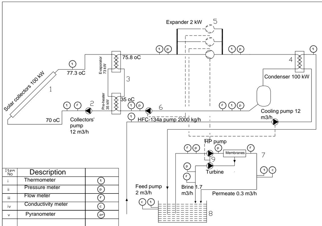
**Figure 1.** Schematic diagram of the prototype system
